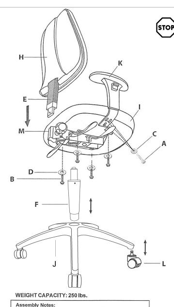
During assembly, hand tighten screws. Only when all screws are in place, you may then tighten all screws completely.
